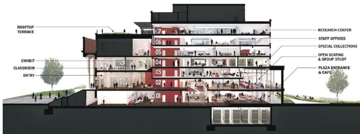
Building section illustrating the programming of floors within the library to incorporate more study and collaborative spaces from the Gorgas Library Master Plan by Shepley-Bulfinch.
