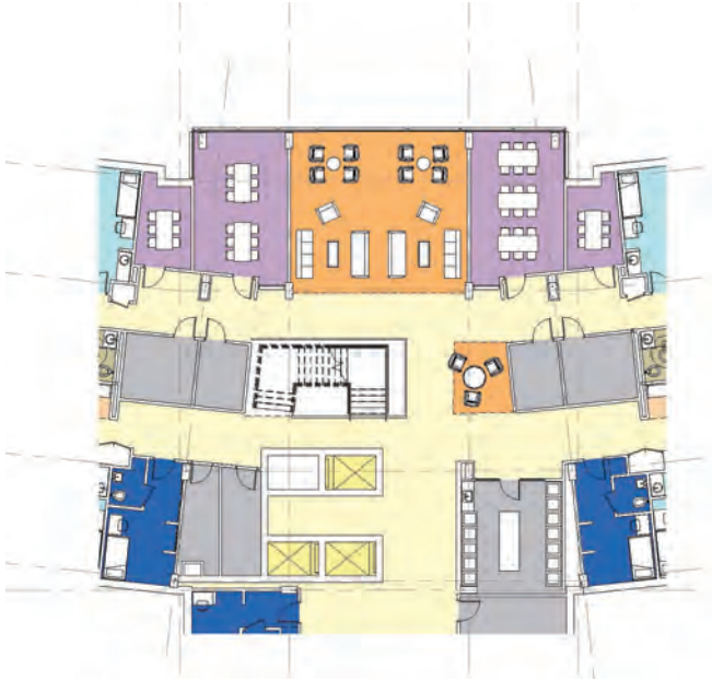
Core Commons - Option03 - Meeting room configuration with centrally located stair
